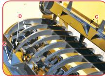
C) New, more aggressive agitators bite into every bale, regardless of condition, to keep it spinning for superior processing. D) New, alternating short and long hoops give you more control to smoothly process any bale, regardless of condition.
