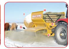
E) More powerful hydraulic motors handle your largest bales. F) Top quality, integrated gear box for right hand discharge. G) 16.5L flotation tires to float over severe conditions. H) Higher, curved sides for better containment during processing. Adjustable loading forks.
