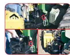
Aq Adaptor Hitch: With the semi-mount receiver installed on your tractor, coupling to your other ag equipment isn't a problem. Simply drop in the Ag Adaptor Hitch. No maneuverability lost.
