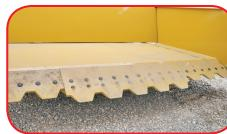
Fill Faster: Dropped center blade section holds the scraper pan down so you get a level cut. Available serrated blades penetrate with more force per inch of blade for faster filling with less demand on your tractor, even in hard packed ground.
