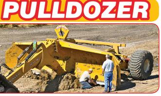
**TRENCH:** All models are available with the retractable trencher. Will simultaneously cut a trench up to 24" deeper than the blade. Quickly drain an area without moving as much dirt. For more information on Pulldozers and Transformers ph Bridgeview at 306-745-2711
