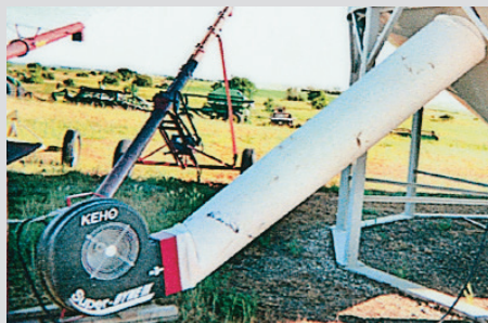
KEHO fans and Air Tubes to provide portability and easy hookup
