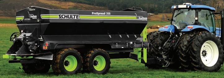
The FLAT BAR chain conveyance provides accurate metering of all types of products. Even inconsistent size product such as biosul is consistently brought to the rear of the bin ensuring metering accuracy.
