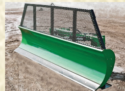
Loader Blades: 6' to 14 widths. Hydraulic or manual angling. Optional screen & end plates.
