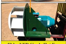
50 hp VFD Single Hot Fan 21 kw -28 hp VFD Cold Fan
