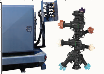
Example boomless nozzle assembly on a service utility truck.
